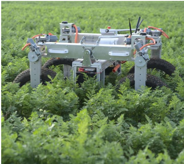
Laser-based weeding robot
